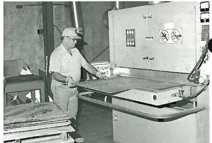
Pruitt feeds an old sign in the sander to remove old paint
